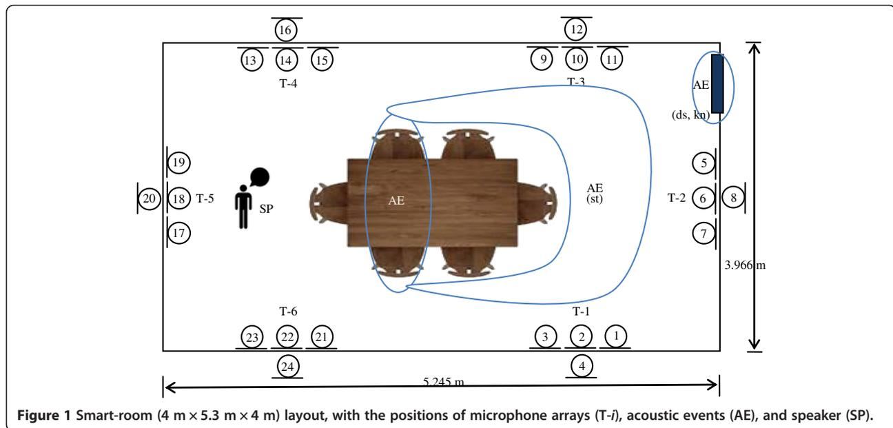
**Figure 1** Smart-room (4 m × 5.3 m × 4 m) layout, with the positions of microphone arrays (T-*i*), acoustic events (AE), and speaker (SP).
