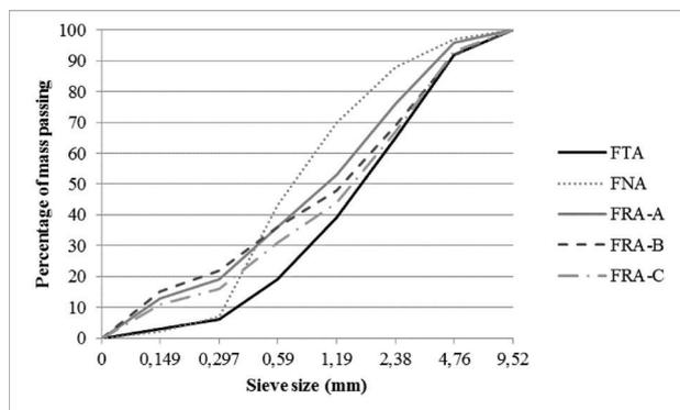
**Figure 2** Particle size distribution of the fine aggregates
