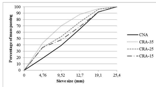
**Figure 3** Particle size distribution of the coarse aggregates
