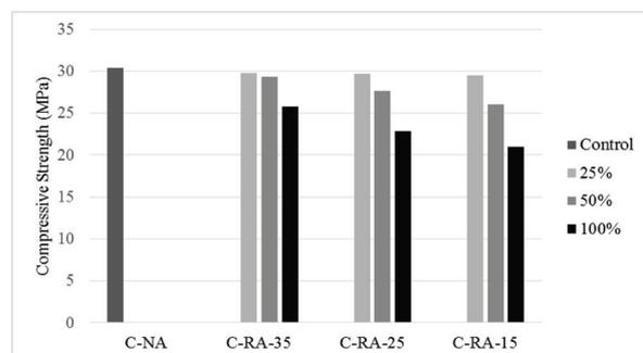
**Figure 6** Compression strength at 28 days of concretes
