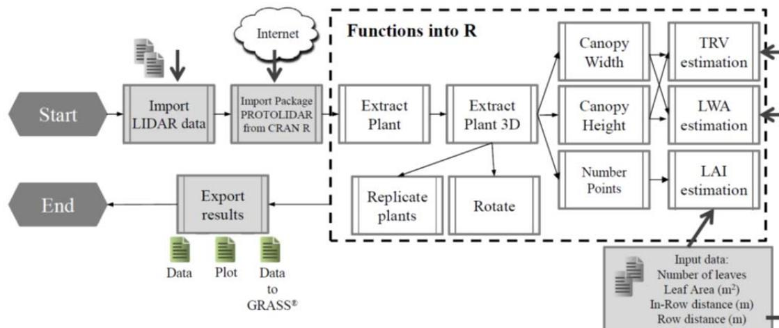
Figure 2. Process diagram of PROTOLIDAR package.
