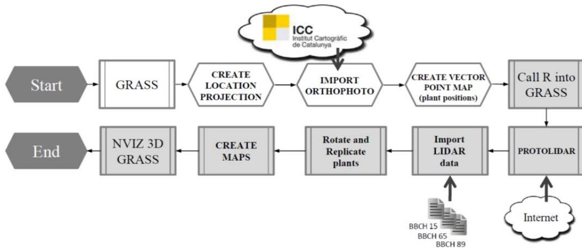
Figure 3. Process diagram of GRASS/R to construct 3D maps
