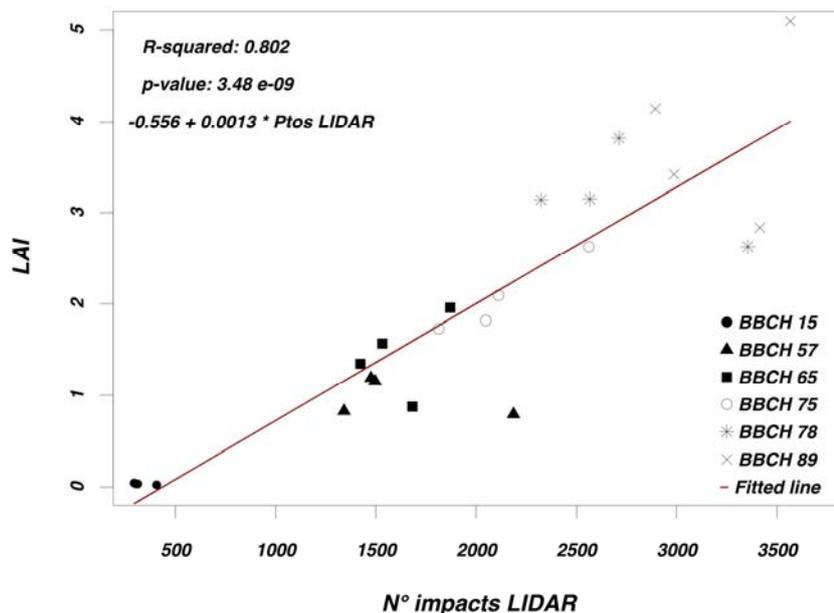
Figure 4. Relationship between the mean number of points of each side of the vine measured with LIDAR sensor in the canopy and LAI.
