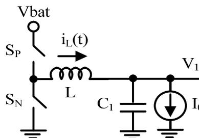
Figure 1. Topology of the basic buck converter.
