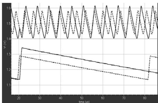
Figure 8. Comparison of static and dynamic hysteresis.
