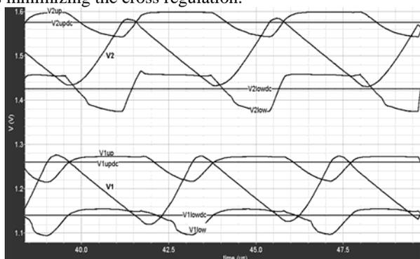
Figure 6. Steady state  $V_1$  and  $V_2$  when load currents  $I_1=I_2=300\text{ mA}$ .
