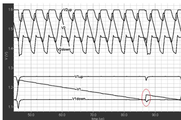
Figure 7. Steady state  $V_1$  and  $V_2$  when load currents  $I_1=10\text{ mA}$  and  $I_2=300\text{ mA}$ .
