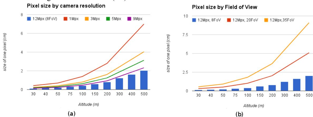
**Figure 1.** Influence of flight altitude, camera resolution and field of view on pixel size
