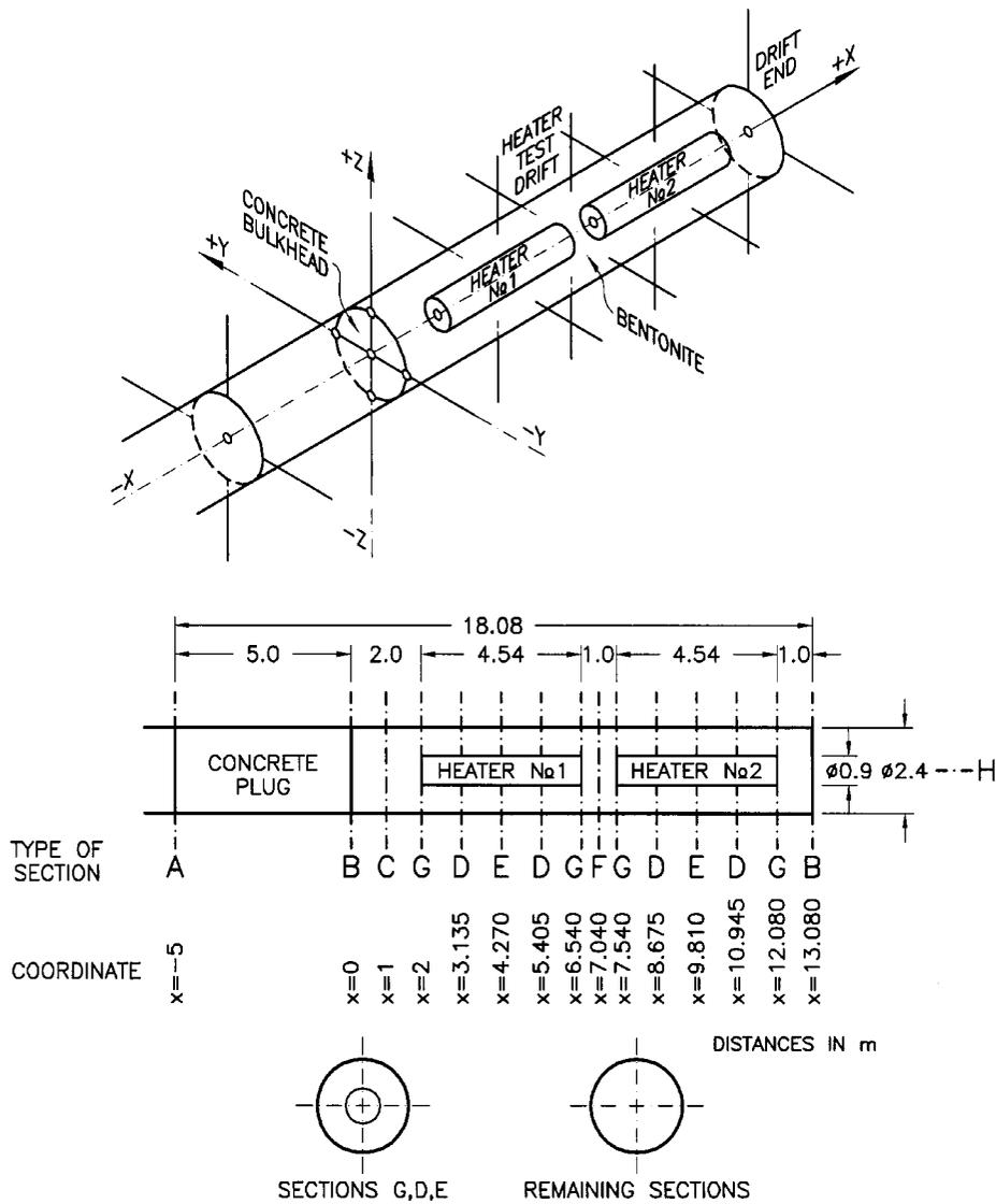
Figure 1. FEBEX test lay out and instrumented sections
