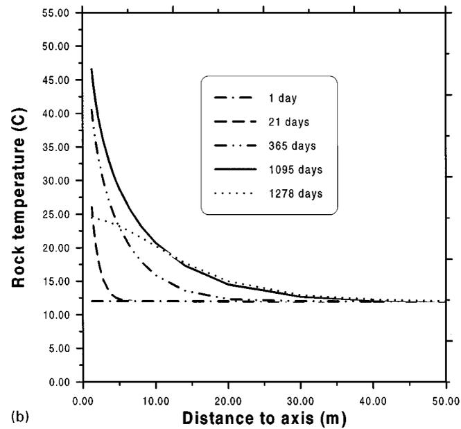
Figure 8. (a) Distribution of temperatures at various times. Near region. THM analysis; (b) Distribution of rock temperature at various times. THM analysis
