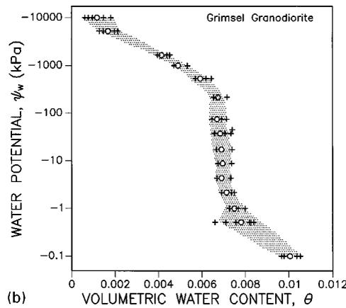
Figure 4. (a) Retention curves for compacted bentonite and granite used in the analysis; (b) Granite retention curve determined experimentally in the laboratory<sup>18</sup>
