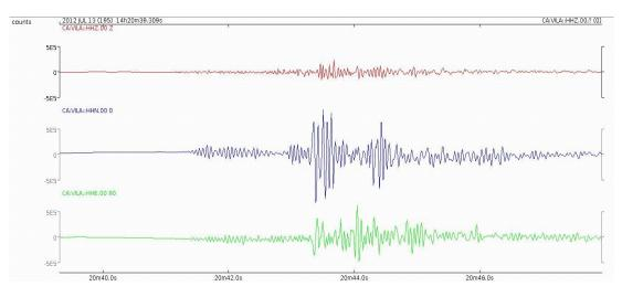
Figure 7 Seismic recordings from VILA station for the local event, magnitude 2.2, on July 13, 2012, in Sant Pere de Ribes (Spain).
