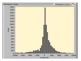
Figure 5 PTP time synchronization drift post deployment (X axis in nanoseconds).
