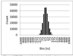
Figure 4 PTP Time synchronization drift on laboratory
