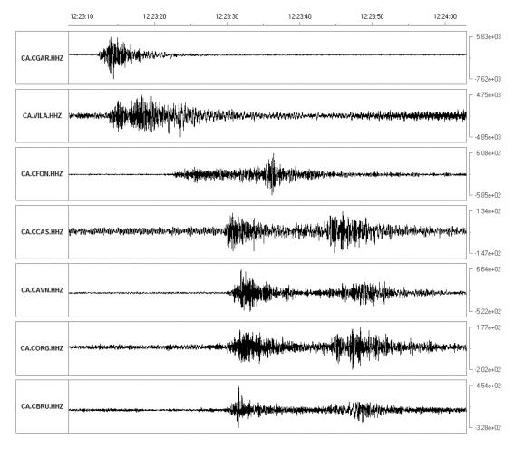
Figure 8 Artificial seismic event recorded by the offshore OBS (VILA) and other seismic stations from Catalan network (CGAR, GFON, CCAS, CAVN, CORG, CBRU), on May 13, 2013 at 12:23 in Garraf (Spain).
