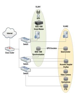
Figure 2 OBSEA network with IEEE 1588 and VLAN setup
