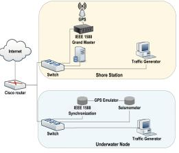
Figure 3 IEEE 1588 Underwater Demonstration Test Setup
