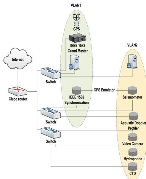
Figure 2 OBSEA network with IEEE 1588 and VLAN setup
