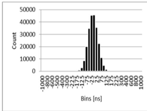
Figure 4 PTP Time synchronization drift on laboratory
