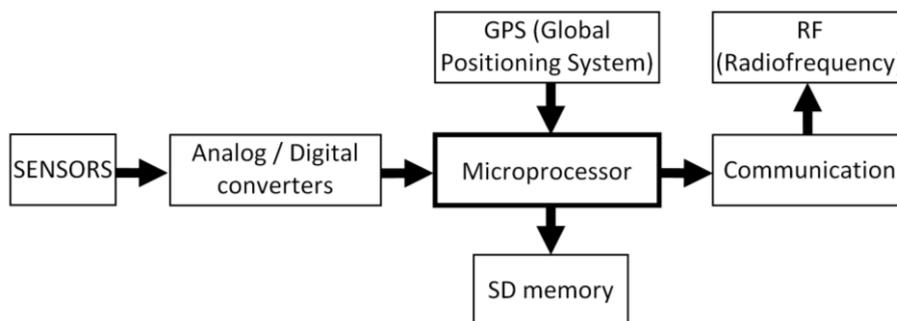
Figure 1. Block diagram of the acquisition system
