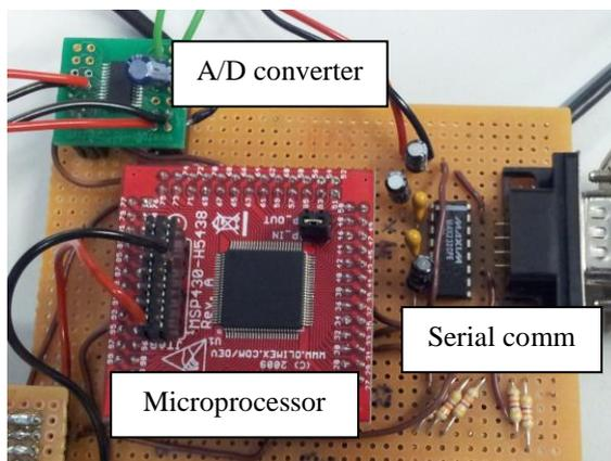
Figure 2. Prototype of acquisition system
