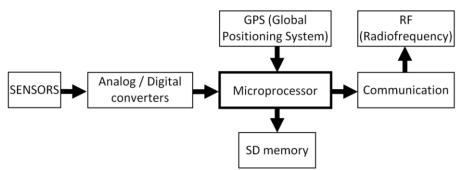
Figure 1. Block diagram of the acquisition system
