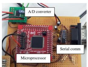
Figure 2. Prototype of acquisition system
