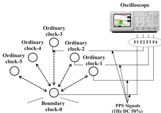
Figure 2 Illustration of the offset measurements setup
