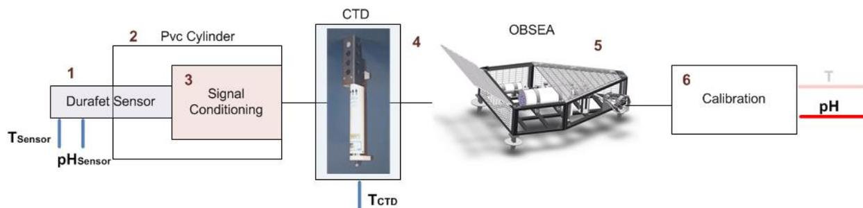
Figure 1 Measurement System
