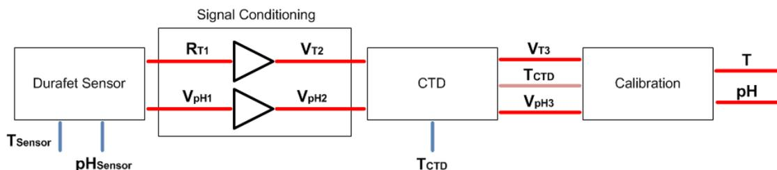
Figure 2 Description of the measurement system
