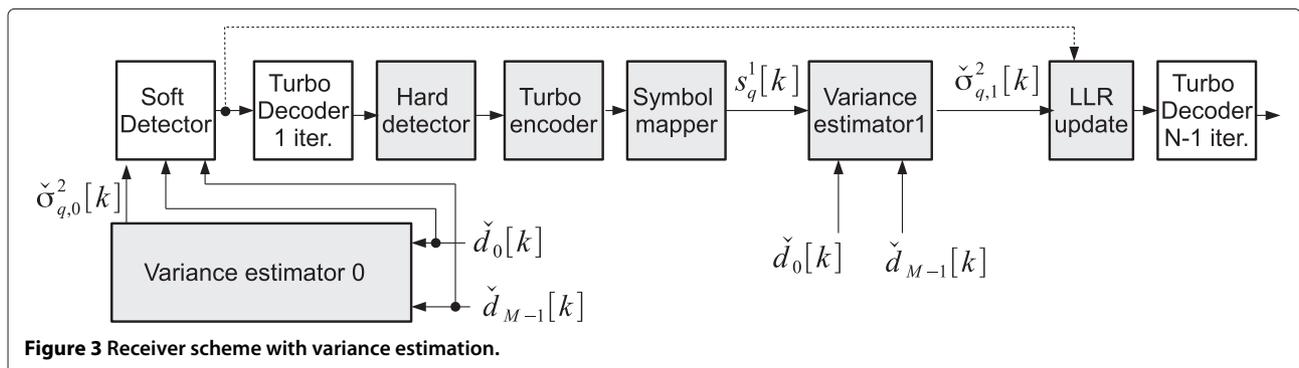
Figure 3 Receiver scheme with variance estimation.
