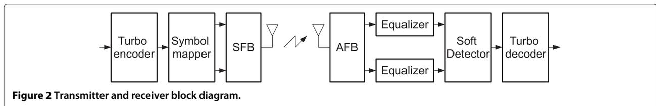
Figure 2 Transmitter and receiver block diagram.
