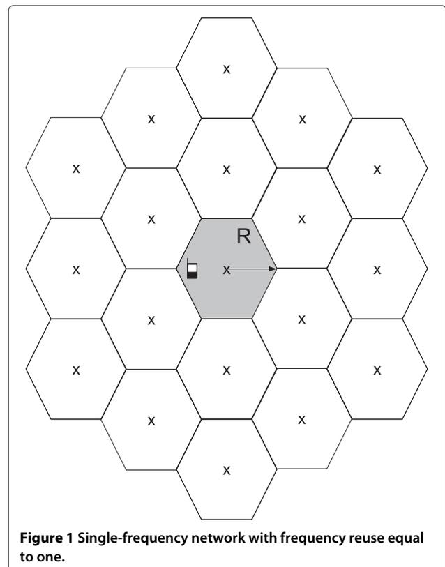
**Figure 1** Single-frequency network with frequency reuse equal to one.
