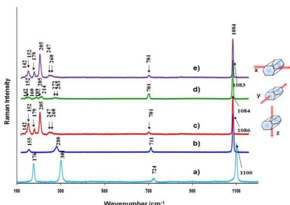
Fig. 2. Raman spectra of the reference minerals: a) dolomite (CaMg(CO<sub>3</sub>)<sub>2</sub>); b) calcite (trigonal CaCO<sub>3</sub>); c),d) and e) are three different orientations (x,y,and z edges) of aragonite (orthorhombic CaCO<sub>3</sub>).
