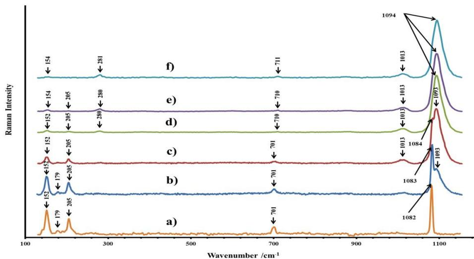
Fig. 4. Raman spectra obtained at different layers of the mollusk cross-section: a) aragonite; b) and c) different concentrations of aragonite mixed with the blue pigment; d) and e) different concentrations of aragonite mixed with the blue pigment and calcite; and f) calcite mixed with the blue pigment.
