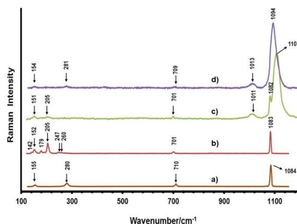
Fig.5. a) Raman spectrum of calcite mineral; b) informative sum of the Raman spectra (x,y and z) of the aragonite mineral; c) and d) are the Raman spectra of the colored areas of the conch and the mussel shells respectively.
