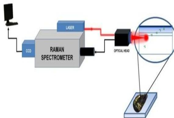
Fig. 1. Scheme of a fiber optic Raman system
