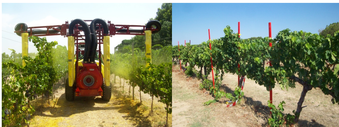
Fig. 1. IRIS multi row sprayer (Ilemo Hardi, S.A.U.) used during the field trials (left); detail of collector's placement on the crop (right).
