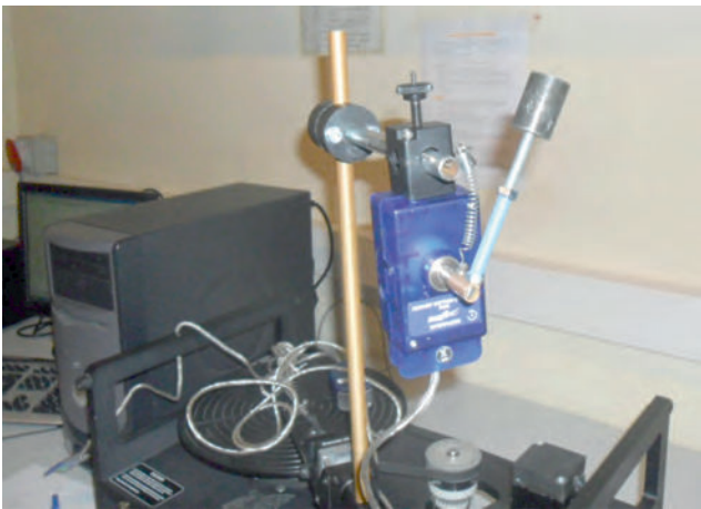
Fig. 7. External disturbance: Second position modification of pendulum accessory, at 35sec. (see Fig. 8)
