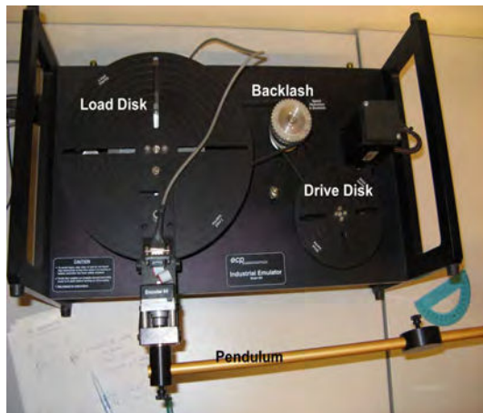
Fig. 1. Basic pendulum assembly control (Model M220) of ECP systems company (ECP 2003).
