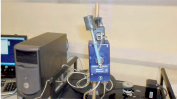
Fig. 6. External disturbance: First position modification of pendulum accessory, at 17sec. (see Fig. 8)
