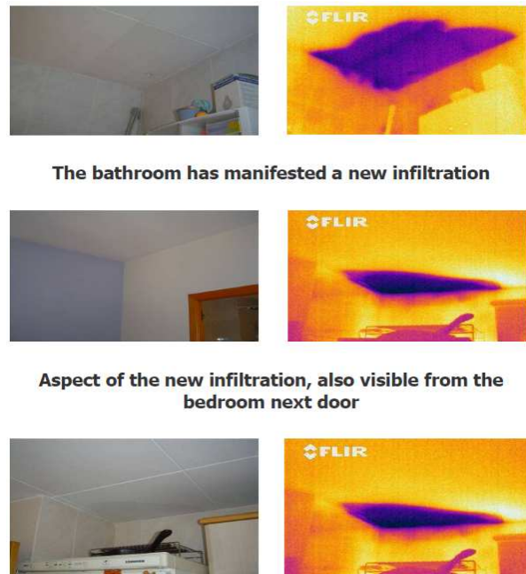
New moisture infiltration that has appeared in the kitchen
