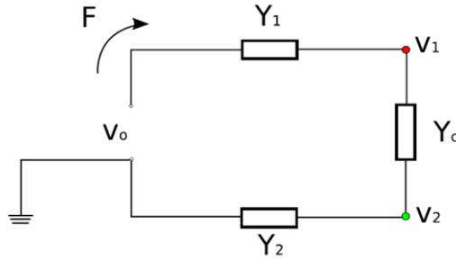
Figure 1 – Circuit equivalent to a double wall
