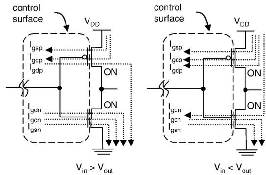
**Fig. 1** CMOS inverter with its input signal floating owing to full open. Voltage at input node assumed to be in a range turning on both transistors. Otherwise, gate-to-channel components would not exist
