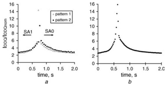
**Fig. 4** Time-dependent behaviour of experimental defective device (HP-82000) and of defective device for patterns 1 and 2
