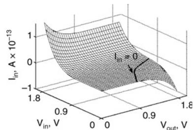
**Fig. 2** Resulting sum of all leakage gate current components ( $I_{in}$ ) at floating input of defective CMOS inverter illustrated in Fig. 1 for a technology with  $t_{ox} = 30\text{Å}$  and minimum size for transistors (curve level for  $I_{in} = 0$  illustrated)
