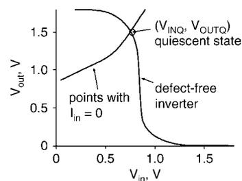
**Fig. 3** Quiescent state of defective inverter obtained from intersection between pairs ( $V_{in}$ ,  $V_{out}$ ) causing  $I_{in} = 0$  and DC transfer characteristic of defect-free inverter
