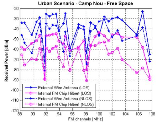
Fig.7 Free space measurement of the power received by the external wire and internal FM Chip Hilbert antennas in the urban scenario.
