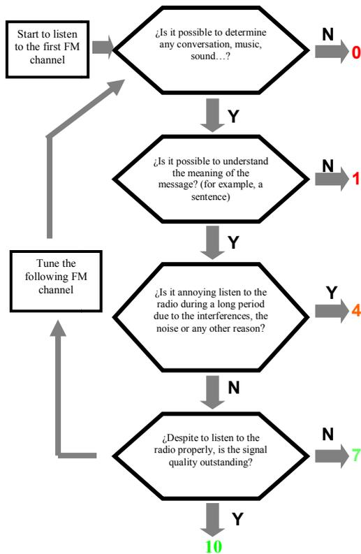
Fig.10. Procedure for evaluating the signal quality indicator.
