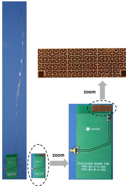
Fig.1 External wire and internal FM Chip Hilbert antennas attached to a typical smart phone platform, [5-6]
