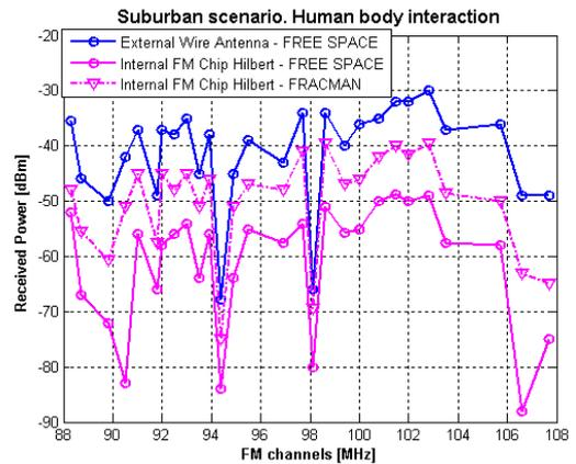
Fig.8 Free space measurement of the power received by the external wire and internal FM Chip Hilbert antennas in the suburban scenario. Together with the power received by the internal FM chip Hilbert antenna under the FracMan condition.
