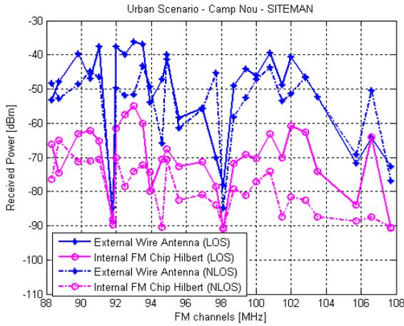
Fig.9. Measurement of the power received by the internal FM Chip Hilbert and external wire antennas under the SiteMan condition in the urban scenario.
