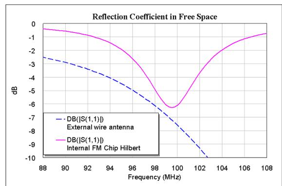
Fig. 4 Free space measurement of the reflection coefficient for the internal FM Chip Hilbert and external wire antennas.
