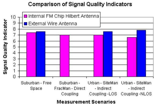
Fig.11. Signal quality indicators which quantify the quality of the FM radio signal received by the internal and external antennas.
