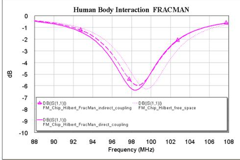
Fig.5 Measurement of the reflection coefficient for the internal FM Chip Hilbert antenna performed under the FracMan condition.
