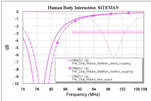
Fig.6. Measurement of the reflection coefficient for the internal FM Chip Hilbert antenna performed under the SiteMan condition. The dotted line at -3dB corresponds to the FM band.
