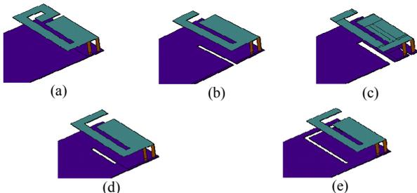
Fig. 2. 3D views of the proposed designs. (a) PIFA without slots, (b-c) PIFA with one open slot or two, (d-e) PIFA with the central slots. [6],[24]
