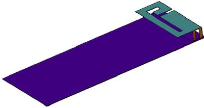
Fig. 1. 3D view of the PIFA dual band. Ground plane is 100 x 40 mm<sup>2</sup> and PIFA is 40 x 15 x 6 mm<sup>3</sup>. [6],[24]
