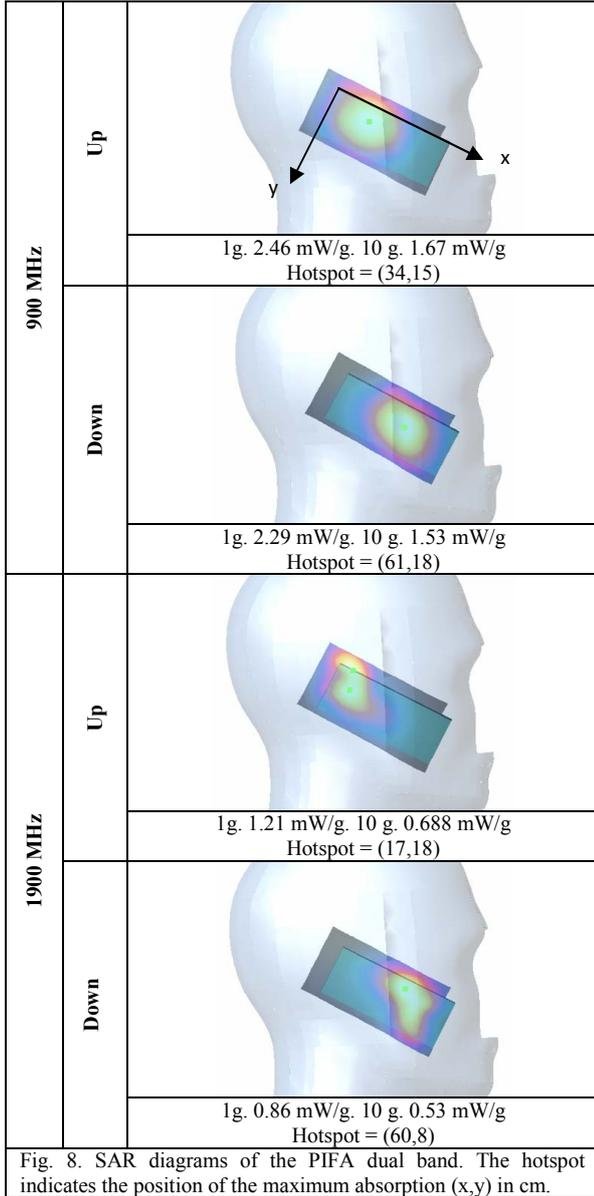
Fig. 8. SAR diagrams of the PIFA dual band. The hotspot indicates the position of the maximum absorption (x,y) in cm.
