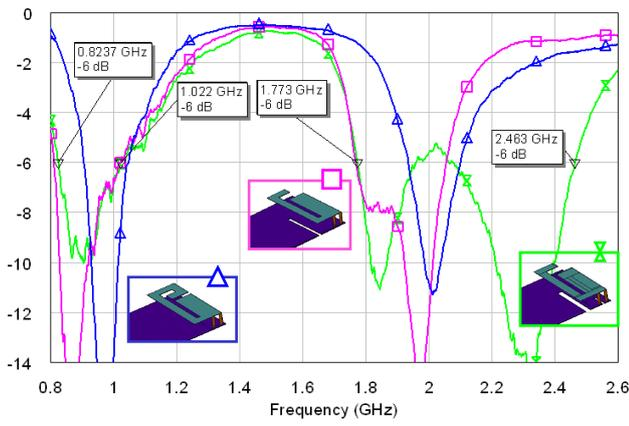
Fig. 4. Comparison of the measured reflection coefficient between PIFA dual band and PIFAs using open slots.
