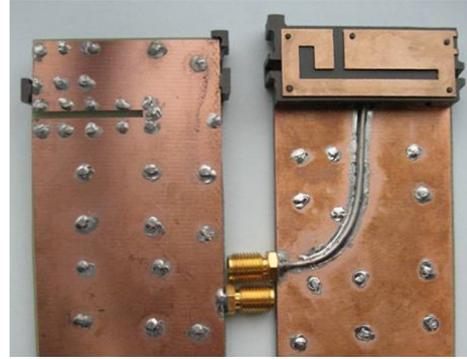
Fig. 3. Prototypes have been constructed. Left: Ground plane configuration for Fig. 2-b. Right: PIFA antenna.
