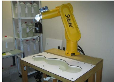
Fig. 7. SAR experiments have been measured with DASY4.
