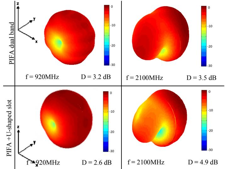
Fig. 6. 3D radiation patterns corresponding to the PIFA dual band and PIFA with U-shaped slot.
