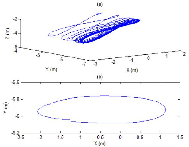
Fig. 21. Buoy model with cable. Orbit of buoy, in m, (a) from 20 s to 600 s and (b) horizontal projection orbit during 1 wave period (7.52 s).
