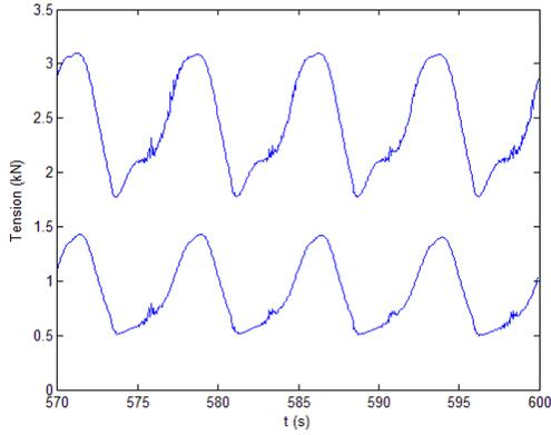
Fig. 16. Buoy model. Detail of instabilities of total (top) and Chain 2 effective tension at EndA at every main period of the series (s).
