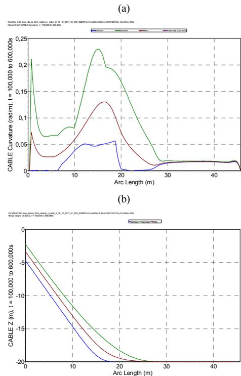
Fig. 22. Buoy model with cable. Results of dynamic simulation of cable as a function of the arc length (m). (a) Range of curvature (rad/m). (b) Range of vertical component z (m).
