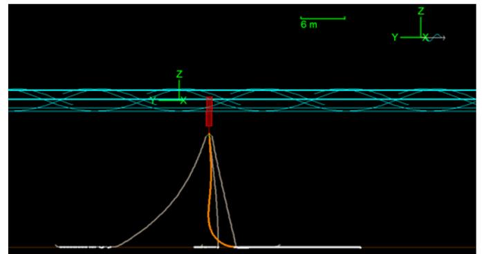
Fig. 9. OrcaFlex 3D-view of Buoy model with cable in a dynamic simulation.
