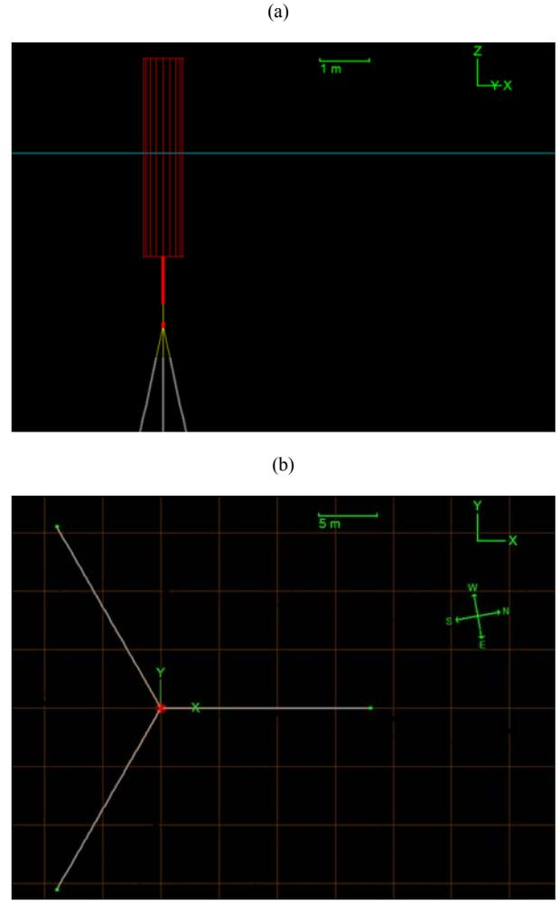
Fig. 7. OBSEA's buoy model without cable on OrcaFlex environment. (a) Vertical view of Spar Buoy type on OrcaFlex environment and links to chains and cable. (b) OrcaFlex plan view of buoy model after the static simulation.
