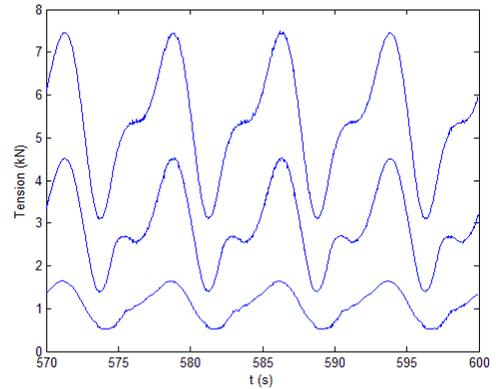
Fig. 17. Buoy model with cable. Detail of temporal evolution (s) of tensions (kN) at EndA. Total, cable and chain 2 effective tension.
