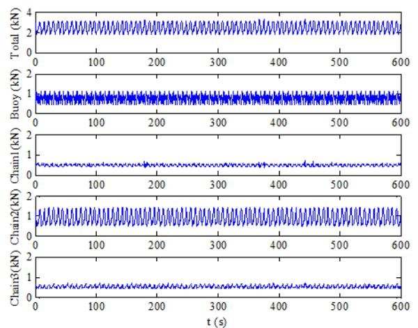
Fig. 14. Buoy model. Temporal evolution (s) of tensions (kN) at EndA. Total effective tension, force of buoy and effective tensions of chains.
