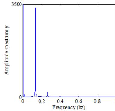
Fig. 12. Buoy model. FFT of relative horizontal position y of buoy, i.e., the amplitude spectrum as a function of frequency (hz).
