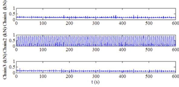
Fig. 15. Buoy model. Temporal evolution (s) of chains' tension (kN) at the anchorage.
