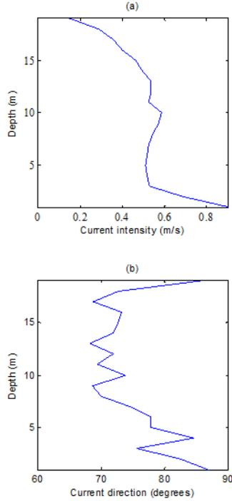
Fig. 5. Current data at 21 p.m. (UTC time), 16-12-2011. (a) Current intensity (m/s) and (b) Current direction of advance (degrees) as a function of depth in the vertical axis.
