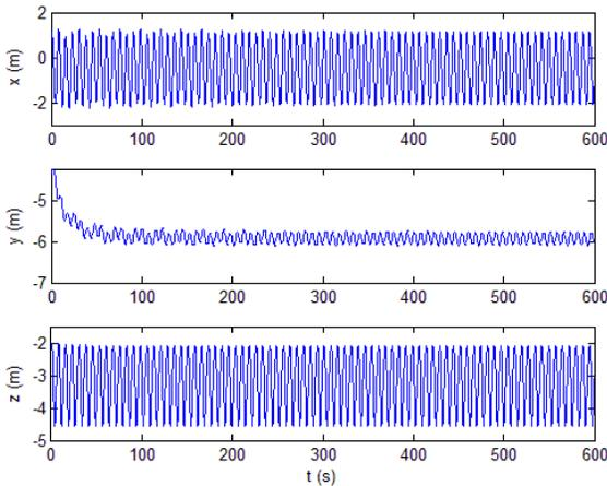
Fig. 19. Buoy model with cable. Temporal evolution (s) of relative positions (x,y,z) of buoy (measured in meters).
