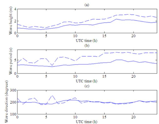
Fig. 4. Wave data series of 16-12-2011 from 0 a.m. to 24 p.m., as a function of UTC time (h) in the horizontal axis. (a) Significant height and maximum height (m), (b) Mean period and peak period (s) and (c) Mean direction and peak direction of advance (degrees), plotted with rigid and dashed lines respectively.
