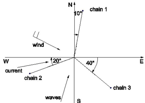
Fig. 8. Schematic plan view (in a NE plan) of Buoy model: chains location and directions of advance of wind, waves and current, 21 p.m. (UTC time), 16-12-2011
