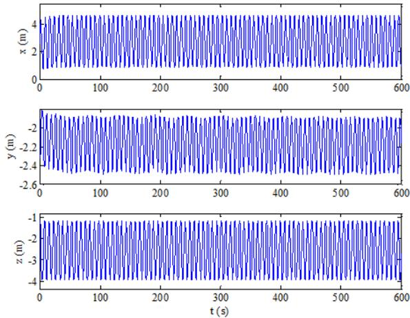
Fig. 10. Buoy model. Temporal evolution (s) of relative positions (x,y,z) of buoy (measured in meters).
