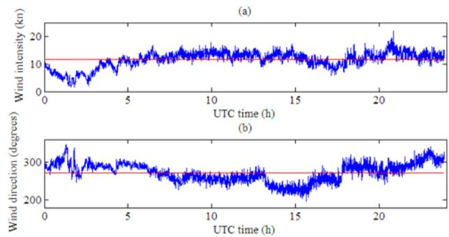
Fig. 3. Wind data series of 16-12-2011 from 0 a.m. to 24 p.m., UTC time. (a) Wind intensity (kn) and (b) wind direction (degrees) as a function of UTC time (h) in the horizontal axis. Red line denotes the corresponding averaged value.
