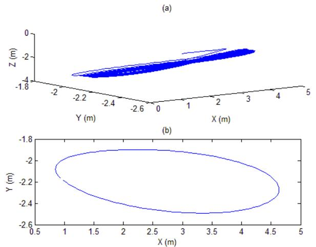
Fig. 13. Buoy model. Orbit of buoy, in m, (a) from 20 s to 600 s and (b) horizontal projection orbit during 1 wave period (7.52 s).
