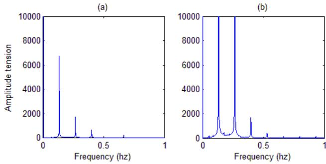
Fig. 18. Amplitude spectrum as a function of frequency (Hz) of total effective tension in Buoy model (a) without cable and (b) with cable.
