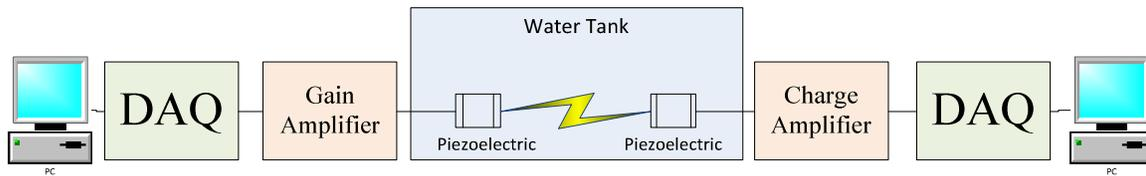
Fig. 2. OFDM communication work bench diagram.
