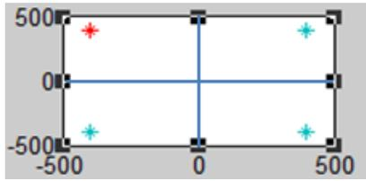
Fig. 3. TX/RX OFDM constellation in loopback mode
