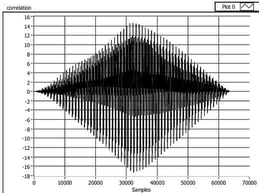
Fig. 8. Correlation between received signal with preamble, and expected preamble.
