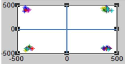
Fig. 4. RX OFDM constellation on air test
