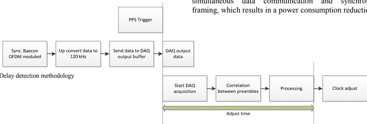
Fig. 9. Delay detection methodology
