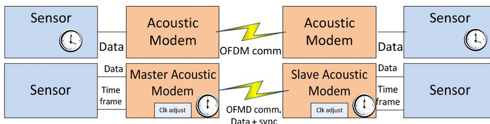
Fig. 1. Actual commercial modems functionality. (up). Acoustic modem with synchronization capabilities (down).
