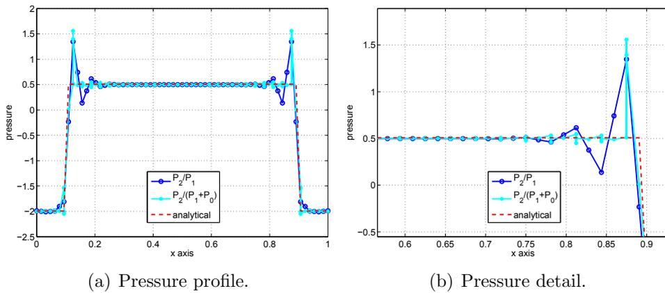
Figure 3: Pressure profile for Hood-Taylor finite element.
