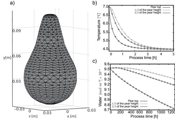
Figure 1: a) 3D geometry and FEM mesh; b) & c) Comparison of solutions achieved by FEM (continuous lines) and ROM for the validation experiment at three different spatial points.
