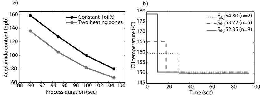
Figure 3: a) Acrylamide content versus process duration for optimally designed 1 and 2 heating zones. b) Optimal operation profiles (oil temperatures) using different numbers of heating zones ( $t_{final} = 95$  s).
