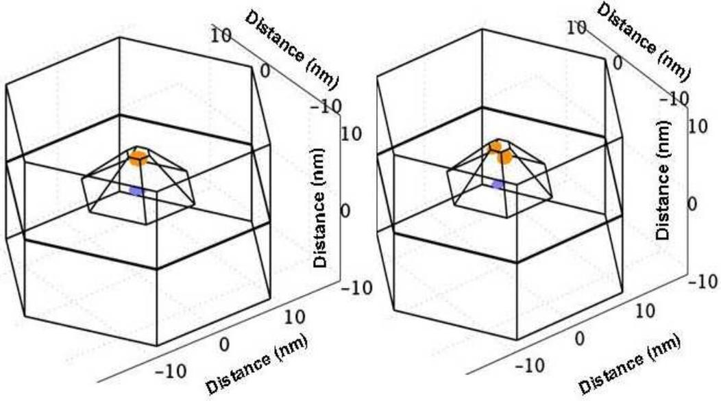
Figure 5: (Color online) Probability distributions of ground and first excited states of electrons (holes) in an AlN/GaN quantum dot with piezoelectromechanical effects. Notice that the piezoelectromechanical effects bring the localization of electron wavefunctions to the top of the dot and hole wavefunctions to the bottom of the dot.
