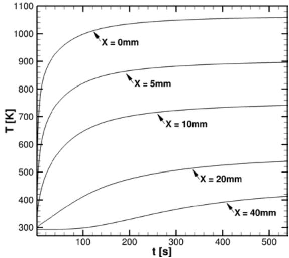
Figure 6: Evolution of temperature on the front face
