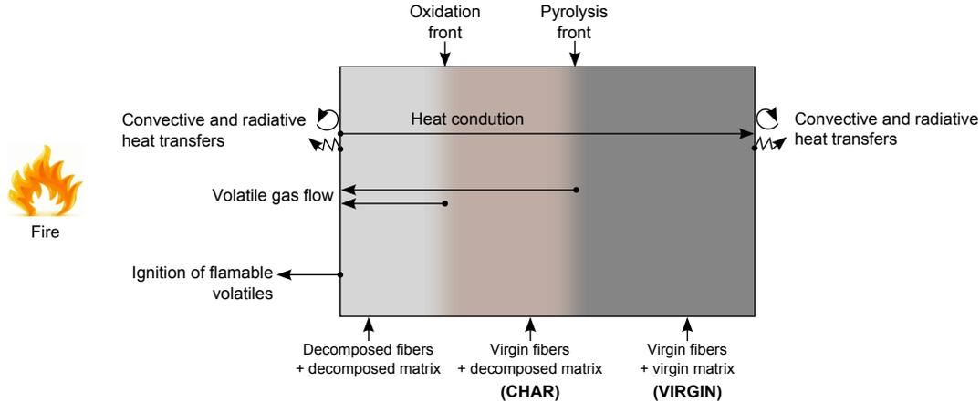
Figure 1: General scheme of the reaction processes in the through-thickness direction of a decomposing composite during fire exposure
