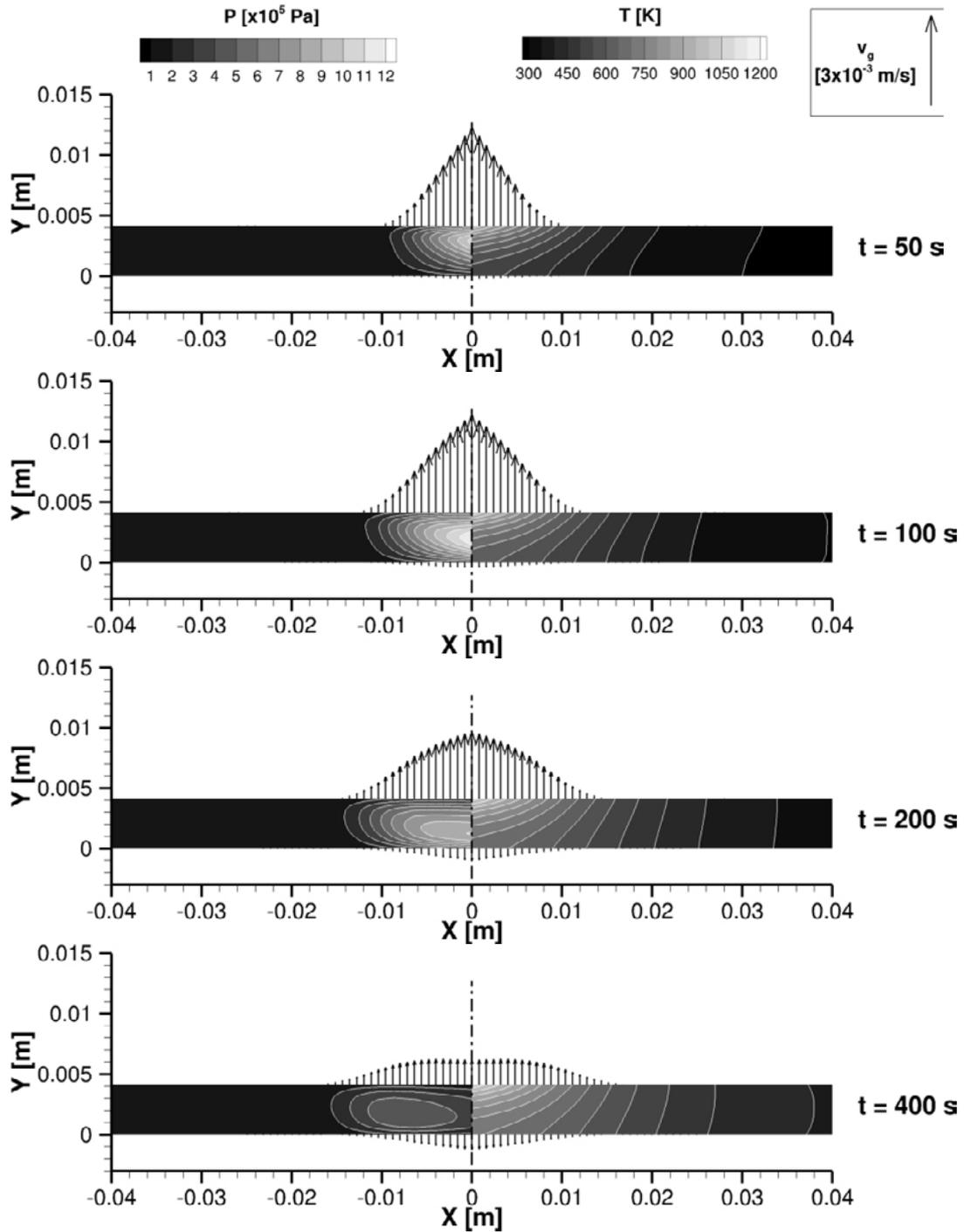
Figure 2: Temperature (right hand side) and pressure (left hand side) distributions associated with averaged gas velocities on surfaces extracted at different times
