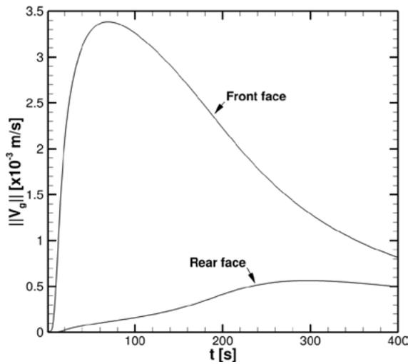
Figure 5: Norm of averaged gas velocity at the front and rear face at  $X = 0mm$
