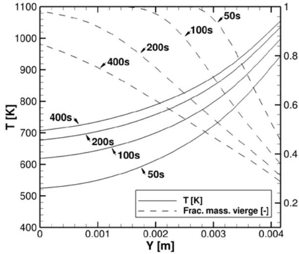
Figure 3: Temperature and virgin mass fraction along the symmetry axis
