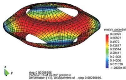
**Figure 3:** electric potential contour plot of the deformed configuration at  $|\phi| = 0.64$  at the rim of the top and bottom hole
