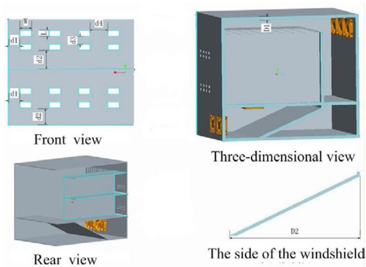
**Figure 3:** Schematic diagram of an airborne cabinet
