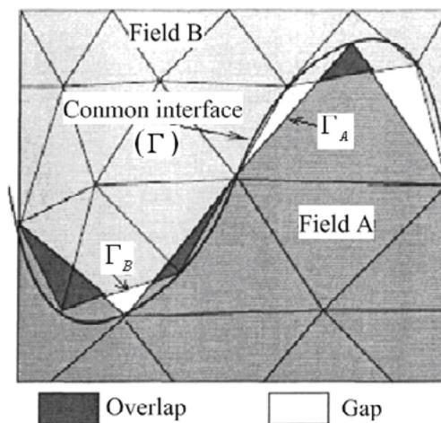
**Figure 1:** Schematic diagram of the grid mismatch
