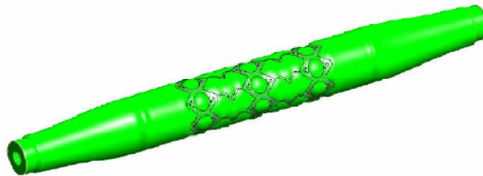
**Figure 7:** Final shape of the stent and balloon after the expansion process.
