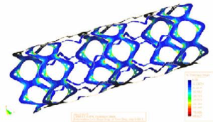
**Figure 8:** Plastic strain distribution in the stent material after the angioplasty.
