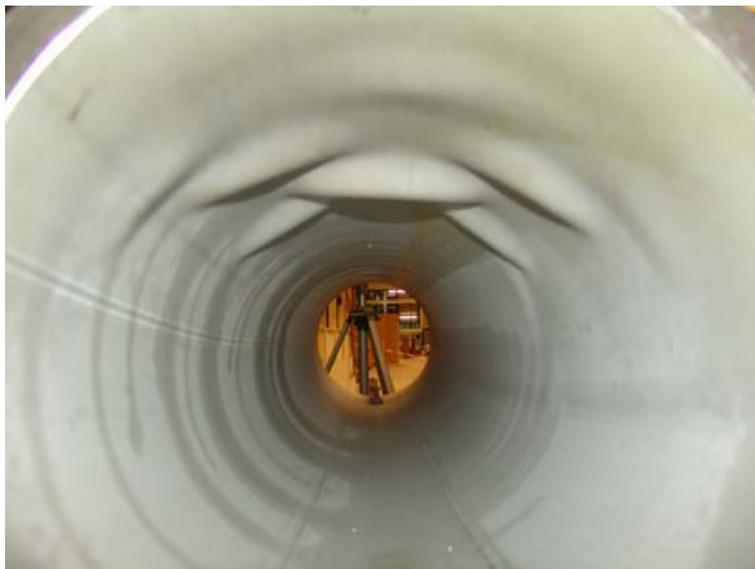
**Figure 4:** Typical form of liner wrinkling following completion of test [1]
