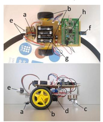
Fig. 2. Top and front view of the mobile robot
