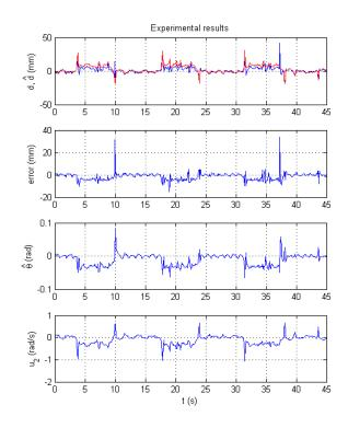
Fig 3. From top to bottom: (1) Comparison between the distance measured, in red, and observed, in blue. (2) Error between measured and observed distance. (3) Observed angle. (4) Control action  $u_2$ .
