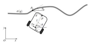
Fig. 1. Two-wheel differential drive mobile robot
