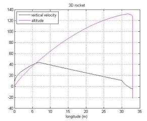
FIG. 4: 3D rocket trajectory in meters (purple) and sinking rate in meters per second (black).
