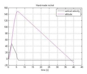
FIG. 3: Hand-made rocket trajectory in meters (purple) and sinking rate in meter per second (black).
