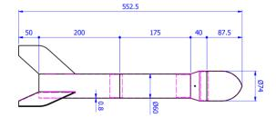
FIG. 1. Design of the rocket made with Autodesk Inventor.
