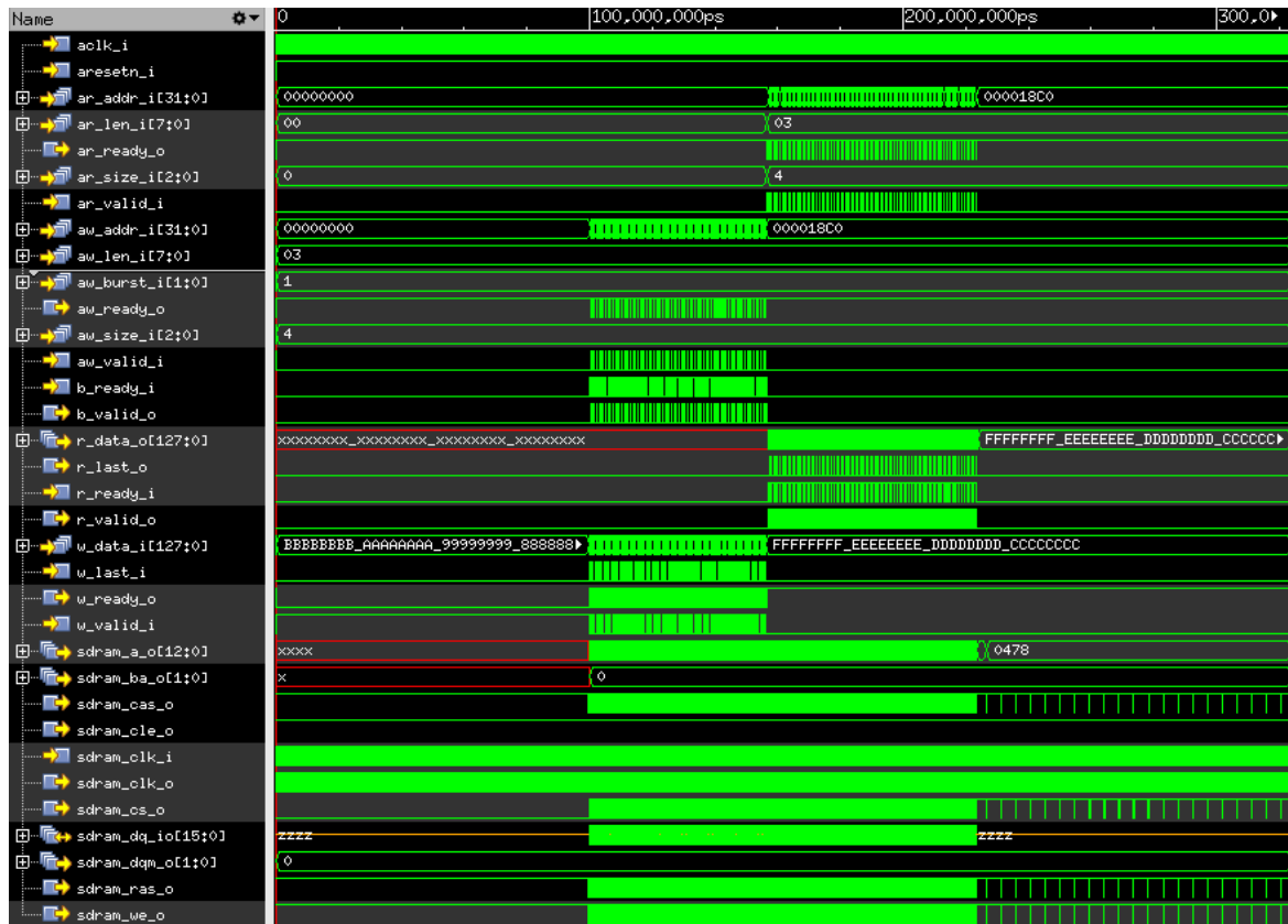
Figure 3.24: Waveforms obtained from the simulation of the AXI SDRAM controller.
