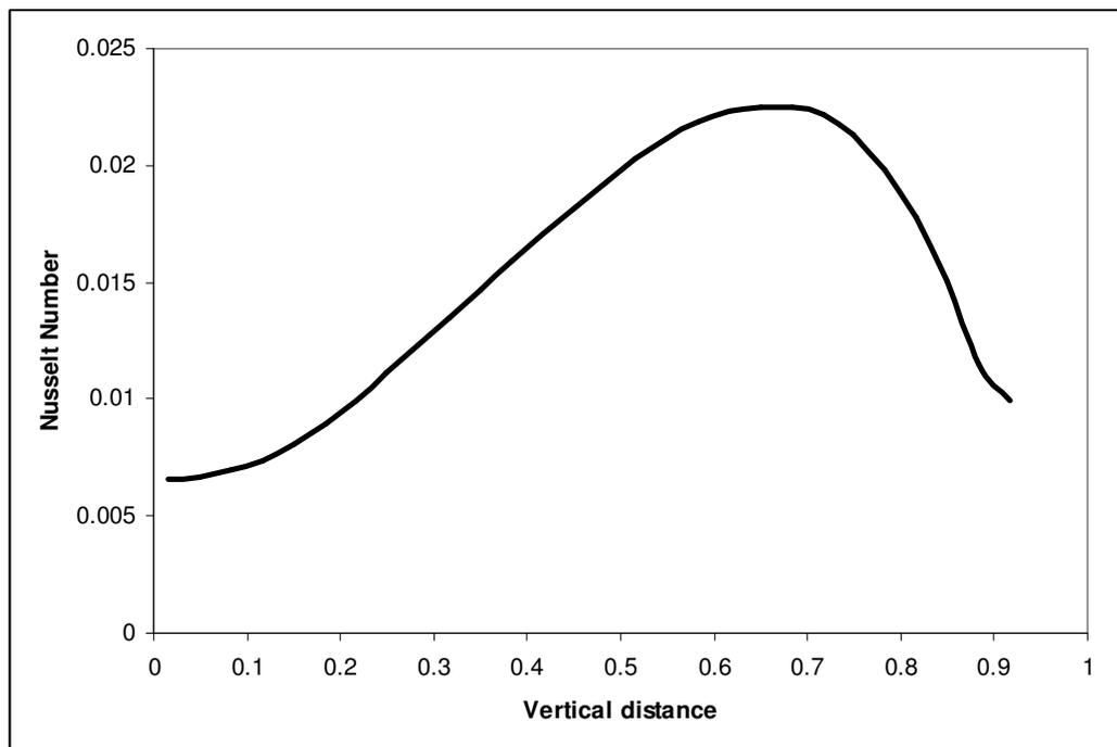
**Figure 4:** Nusselt number in the back wall for the expansion ratio of 1.10
