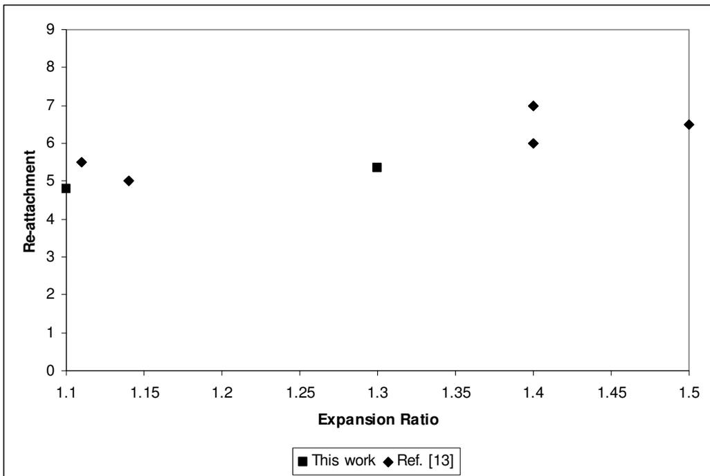
Figure 1: Re-attachment for different expansion ratios
