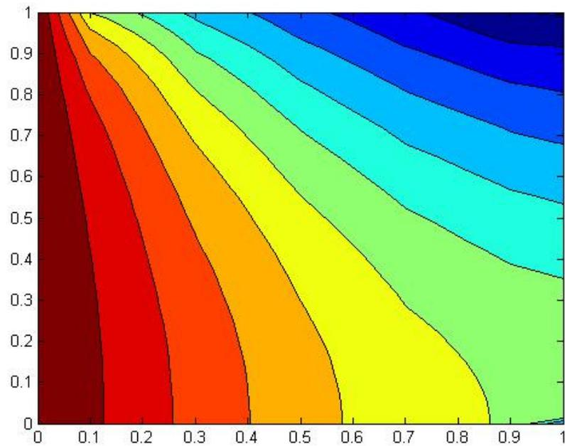
Figure 2: Temperature distribution in the step for an expansion ratio of 1.10
