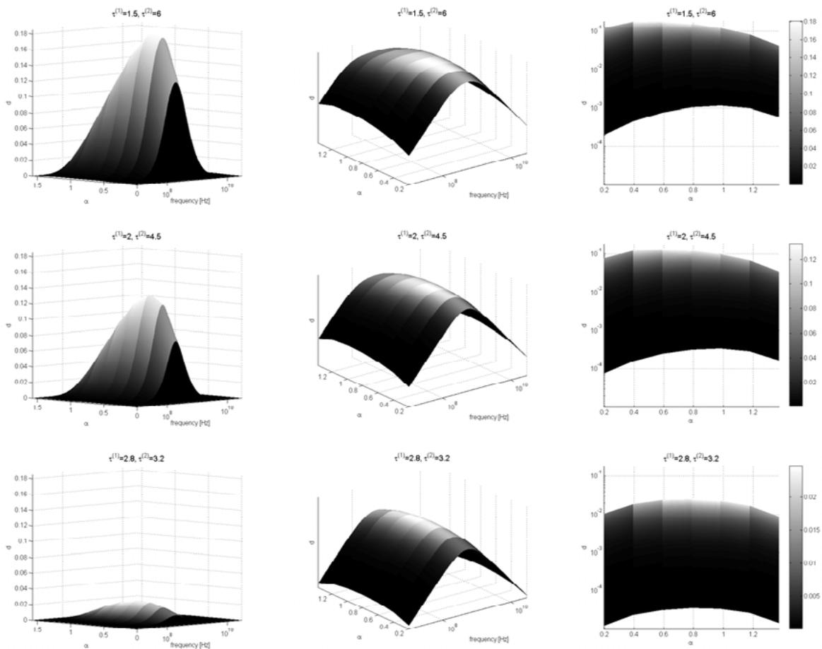
**Figure 3:** Different views of the shear polarization factor  $d$ . Left: as function of frequency and angle  $\alpha$ , middle: logarithmic presentation of  $d$ , right: range of  $d$  in a certain frequency interval in dependence on  $\alpha$ . Pairs of tortuosities – top row:  $\tau^{(1)}=1.5$ ,  $\tau^{(2)}=6.0$ , middle row:  $\tau^{(1)}=2.0$ ,  $\tau^{(2)}=4.5$ , bottom row:  $\tau^{(1)}=2.8$ ,  $\tau^{(2)}=3.2$
