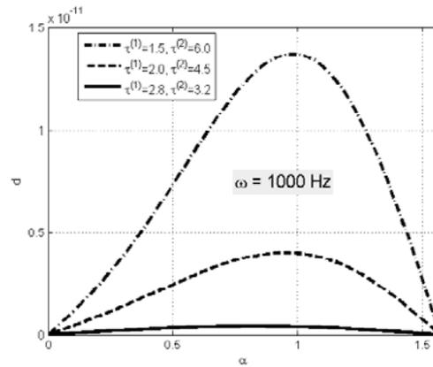
**Figure 4:** Polarization  $d$  as a function of angle  $\alpha$  in Alermoeh sandstein for three pairs of principal tortuosities
