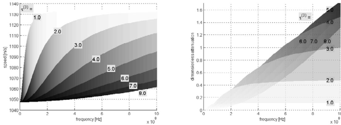
**Figure 1:** Speeds (left) and dimensionless attenuations (right) of the purely transversal wave appearing in Alermoehe sandstone for different values of the principal tortuosity  $\tau^{(3)}$
