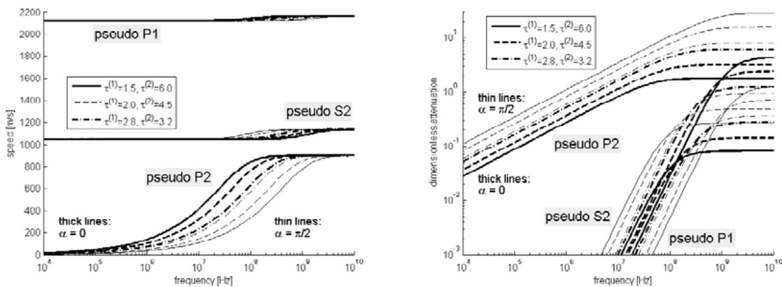
**Figure 2:** Speeds (left) and dimensionless attenuations (right) of the three pseudo waves appearing in Alermoehé sandstein for three pairs of principal tortuosities and two values of angle  $\alpha$
