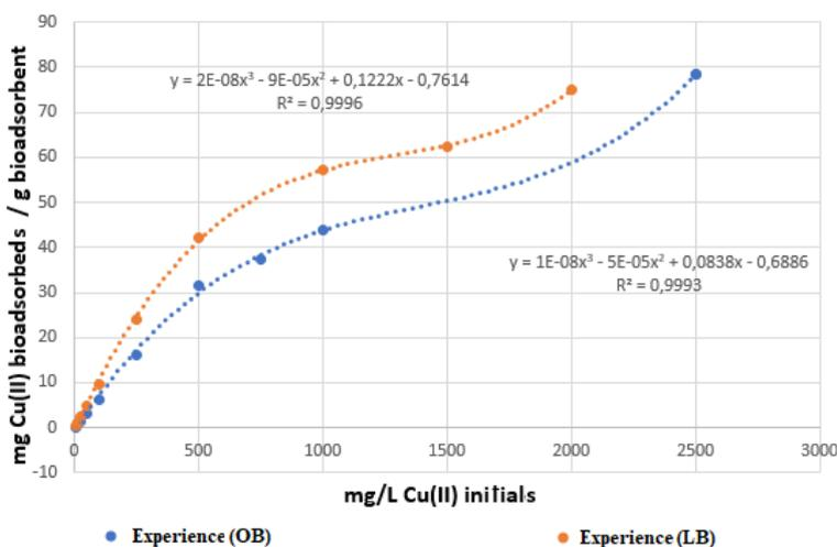
**FIGURE 5. mg Cu(II) bioadsorbeds/ gram bioadsorbent vs [Cu(II)] initial (mg/L)**
