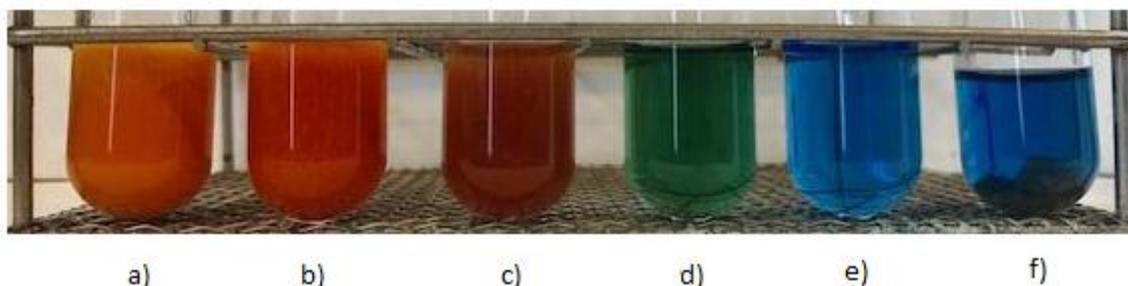
**FIGURE 3. Fehling trial in the different liquid fractions of the chemical treatment of an orange peel: a) first acid attack; b) second acid attack; c) rinse with distilled water; d) alkaline attack; e) rinse with distilled water; f) final bioadsorbent**
