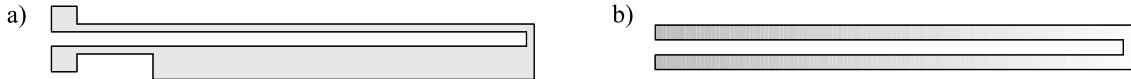
Figure 1: a) Classic shape of MEMS actuator, b) New shape of FGM actuator
