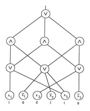
Fig. 1 A monotone alternating boolean circuit C
