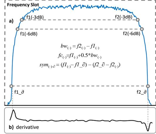
Fig. 2. Relevant points of a QPSK modulated signal
