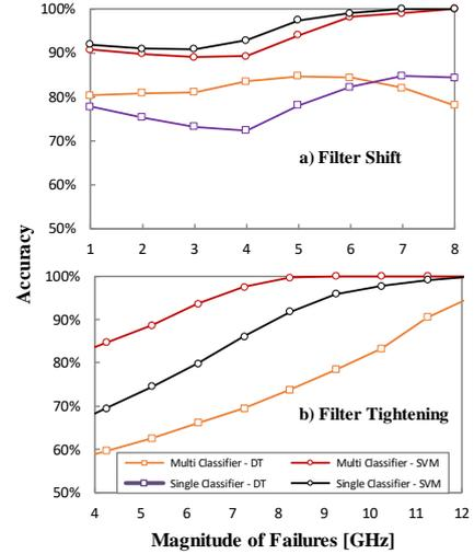
Fig. 7. Average accuracy over N1-N8 of DT and SVM for FS (a) and FT (b).
