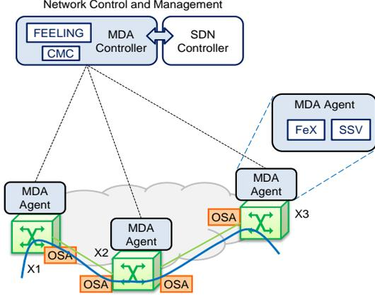
Fig. 1. Architecture for failure identification and localization
