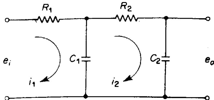
$$\frac{E_o(s)}{E_i(s)} = \frac{1}{(R_1 C_1 s + 1)(R_2 C_2 s + 1) + R_1 C_2 s}$$
