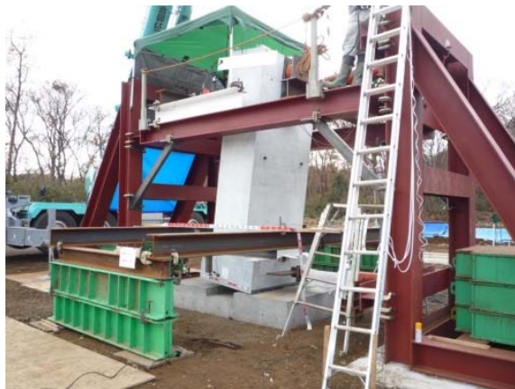
(a) Rocking Specimen under loading (b) Photo of Rocking Specimen under loading
