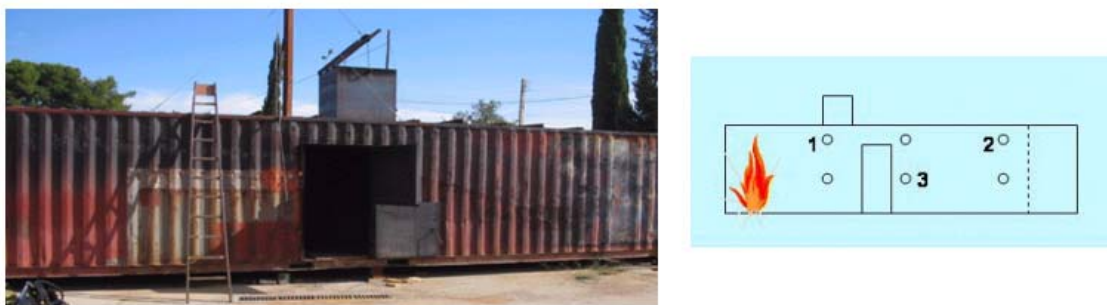
Figure 1. Experimental container with a diagram showing the thermocouple positions.
