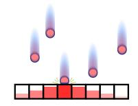
Fig. 5. Graphical representation of the effect of particles impact in a discretized 1-dimensional space
