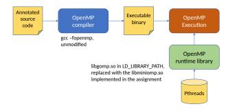
Fig. 1. The OpenMP compilation and execution flow.
