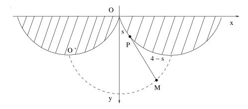
Prove that the path of the suspended mass M is a cycloid, and explain why the period is independent of the oscillations amplitude.
