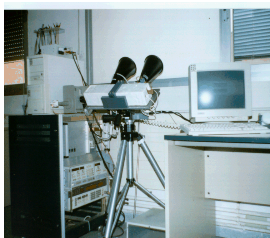
UPC polarimetric radiometer at the D3 antennas-microwaves-radar laboratory.
