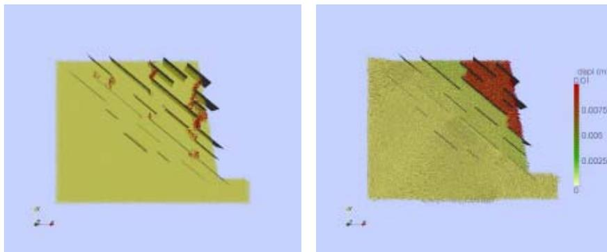
**Figure 5.** Cracks (left) and displacement field (right) induced by strength degradation in the case of a random joint set with a  $40^\circ$  dip angle.
