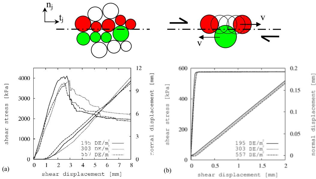
**Figure 2:** Joint contact logic (top) and dependence of the joint behaviour on the model resolution (bottom): Shear displacement curves from direct shear test simulations performed on a joint made up with different numbers of DEs under 1MPa confinement for (a) the classic contact logic and (b) the modified joint contact logic for an interparticle angle equal to 30 degree.
