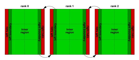
**Figure 2**: Domain decomposition with boundary exchange. Domains are labeled by the rank of the respective compute resource. Each domain (local volume) is extended by the boundaries of its neighbors (halo). A domain is further divided into partitions (indicated by the dashed lines), including the boundary partition(s).
