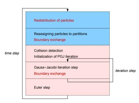
Figure 3: Program flow. Blue boxes indicate pure data management, red boxes contain the actual NSCD algorithm. Tasks involving data exchange with remote compute resources are higlighted in red.
