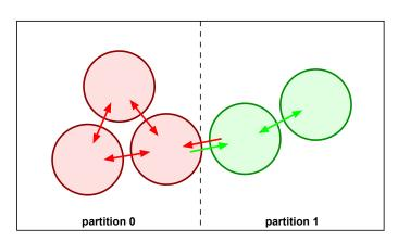
**Figure 1**: Data access pattern at a partition boundary. Particles are uniquely assigned to a partition (indicated by color). Active contacts are shown as lines connecting the particles, write access is marked by an arrow.
