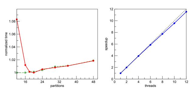
**Figure 4**: (left) The solid red line shows the normalized runtime for 12 cores depending on the number of partitions, the dashed green line represents the normalized calculation time. (right) Speedup for the shared memory system, see text for details.
