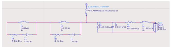
FIG. 2. The photodiode was modelled with a parallel resistance and capacitance and a series resistance and inductance, and our chosen DC-block and inductance are also represented.
