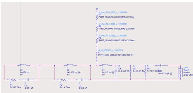
FIG. 4. Laser's equivalent circuit
