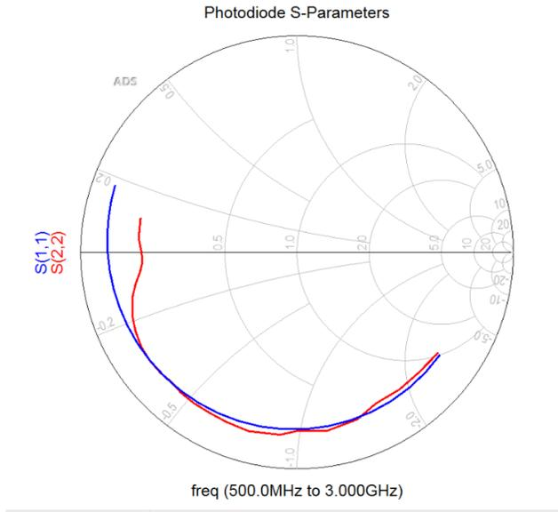
FIG. 3. A representation of the S-parameters of the photodetector, in a Smith chart, the equivalent circuit fits the measurements in the frequencies of interest
