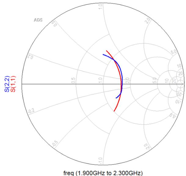
FIG. 5. A representation of the S-parameters of the laser, in a Smith chart, the equivalent circuit fits the measurements in the frequencies of interest
