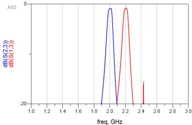
FIG. 6. Transmission for each frequency. The blue band corresponds to the uplink band and the red band to the downlink band.
