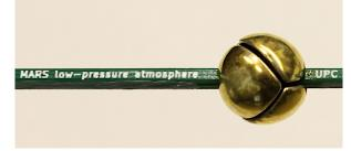
**Fig. 1:** Photograph of the 4-sector spherical sensor (10mm diameter).
