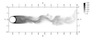
**Fig. 2**: Figure from [4] showing a snapshot of the temperature field in the wake of the sphere for Re1000 obtained from direct numerical simulations of the incompressible Navier-Stokes and energy equations.
