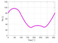
**Fig. 5:** Average Nu number for Re10<sup>4</sup> on the triangle of Fig.3-right as a function of yaw angle.
