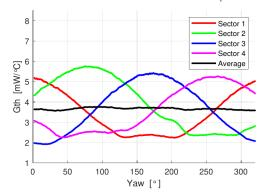
**Fig. 6:** Thermal conductances of each sector, and average value, as a function of Yaw angle for Re1000. Equivalent  $U_{Mars-flow}$  velocity under typical Mars conditions of 65m/s.
